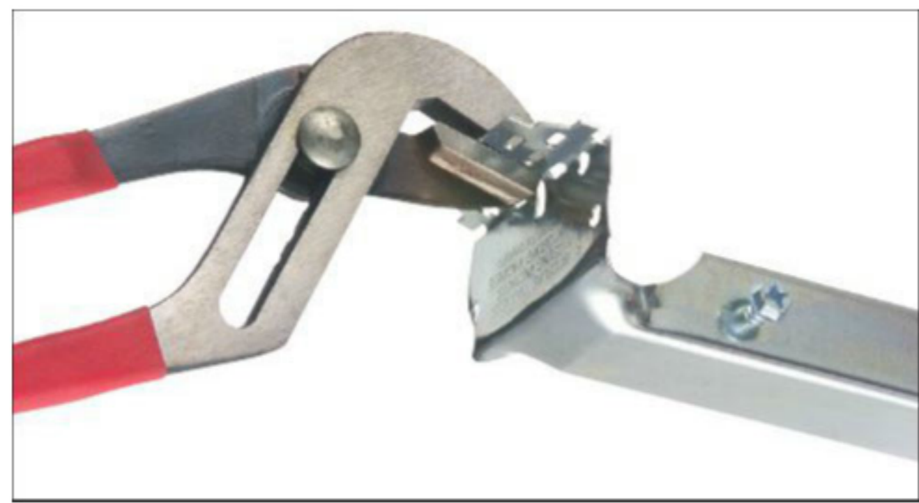
Bracket ends are pre-set for a 1/2" ceiling. For other ceiling depths bend the bracket ends along the appropriate score line.
