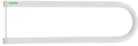
**General Description:** 32W, 22.5 inches MOL, T8 OCTRON XP Extended Performance Curvalume fluorescent lamp, 6 inches leg spacing, 4100K color temperature, rare earth phosphor, 85 CRI, suitable for IS or RS operation, ECOLOGIC
