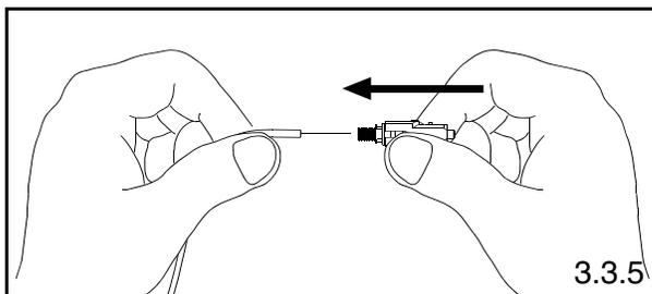
3.3.5 Carefully but quickly insert the bare fiber through the ferrule in a smooth forward motion. The fiber is fully inserted when the buffer bottoms against the rear of the ferrule. The adhesive will begin to set within seconds. **Note: If adhesive oozes out the back of the assembly, you have injected too much. It is critical to the function of the connector that you wipe away all excess adhesive.**
