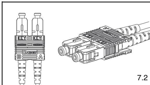
**Note: When making cable assemblies, be sure to follow the correct 'A->B' polarity cross-over between connectors.**
