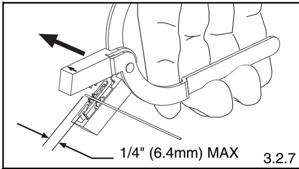
3.2.7 With the buffer stripper provided, strip the buffer.
