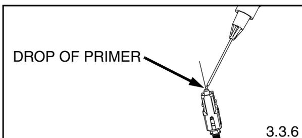
3.3.6 To speed hardening of the adhesive, apply a small drop of primer to the adhesive bead on the ferrule tip using the primer filled syringe. Do not allow the primer to come in contact with the plastic housing of the ferrule assembly. Absorb any primer and unhardened adhesive from the ferrule tip by gently dabbing it with the corner of a lint-free wipe. **Be careful not to break the fiber.**
