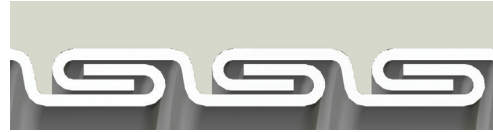
Interlocked Design 1-1/2" through 4" with no bonding wire
