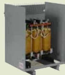
Dual output, phase shifting Harmonic Mitigating Transformers provide extremely low output voltage distortion and input current distortion even under severe non-linear load conditions (Data Centers, Internet Service Providers, Telecom Sites, Call Centers, Broadcasting Studios, etc.). Combining zero sequence flux cancellation with phase shifting treats 3rd, 5th, 7th, 9th, 15th, 17th and 19th harmonics within its secondary windings.
