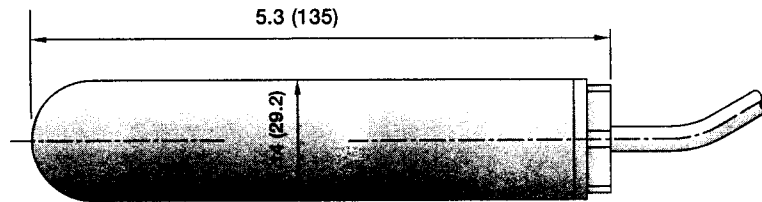
Cylindrical float switch
