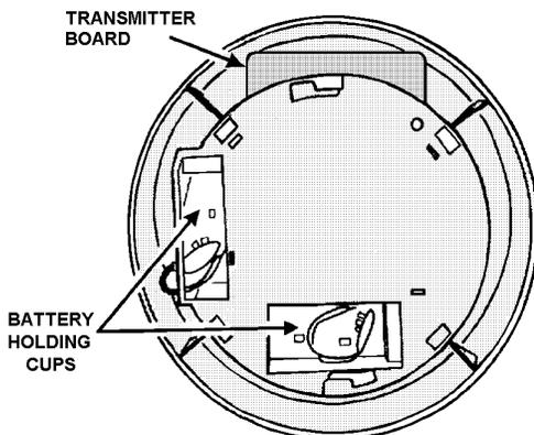
**Step 3. Install batteries.** Connect the two 9-volt alkaline batteries and place them into the battery holding clips.
