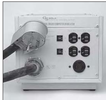
60 Hz, 2000–3000 VA, (4) 5-15R and (1) L5-30R Receptacle
