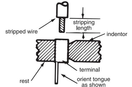
The terminal must be properly installed.
