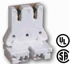
* 22458 Medium Bi-Pin Lamp Holder Floating Action for U-Shape Lamps Low Profile Size Disconnect Feature Guards Against Electric Shock No. 18/20 Gauge 660 Watts Max., 600 Volts
